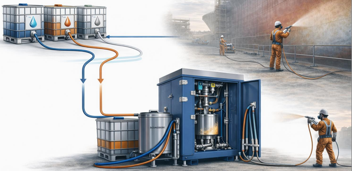
Independent Supply of Base; Curing Agent, and Thinner → Blended Paint
